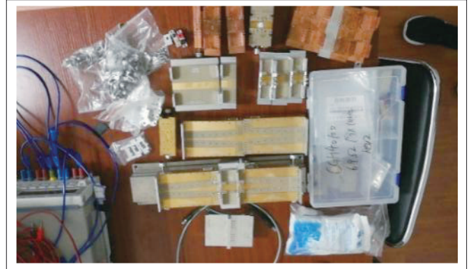
▲ Figure 6. The 6.9 \Omega through reflection line (TRL) measurement fixture
